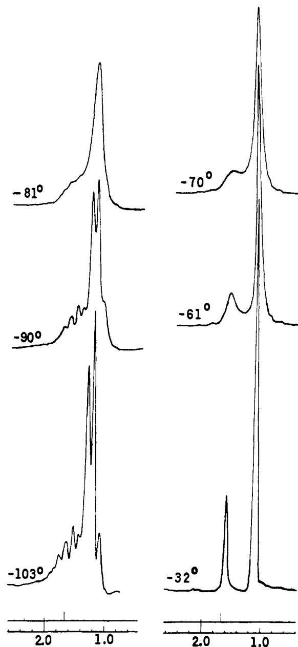
Figure 1. Temperature-dependent pmr spectra of propane exchanging with trace of dimethylcarbenium ion.
